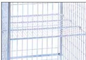
> Standard wire shelf 4.495.03.03 Admissible load: 70 kg. Width 650 mm. Length 730 mm. Space between wires : 16 mm.
