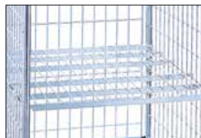
> Reinforced wire shelf 4.495.28.03 Flat steel bars welded to edges. Permissible load : 100 kg. Width 650 mm. Length 730 mm. Space between wires : 37 mm.
