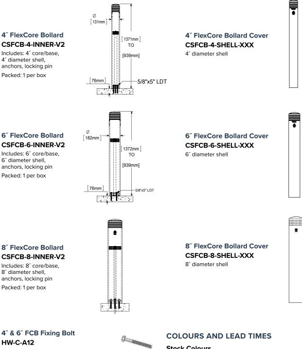
**HW-C-A12**  $\frac{1}{2}$  x 6" self tapping concrete screw
